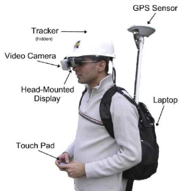
Fig. 1. Overview of the developed AR hardware framework.
