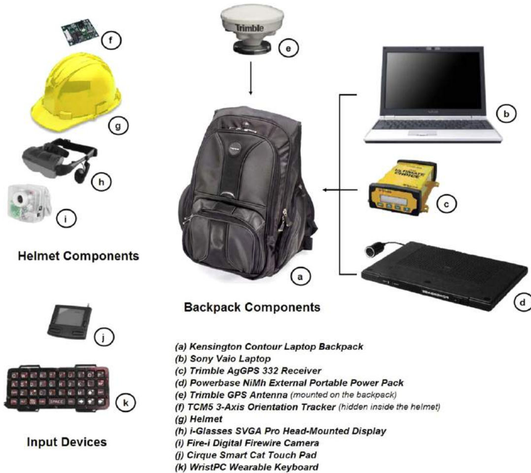
Fig. 2. Hardware components of the AR system.
